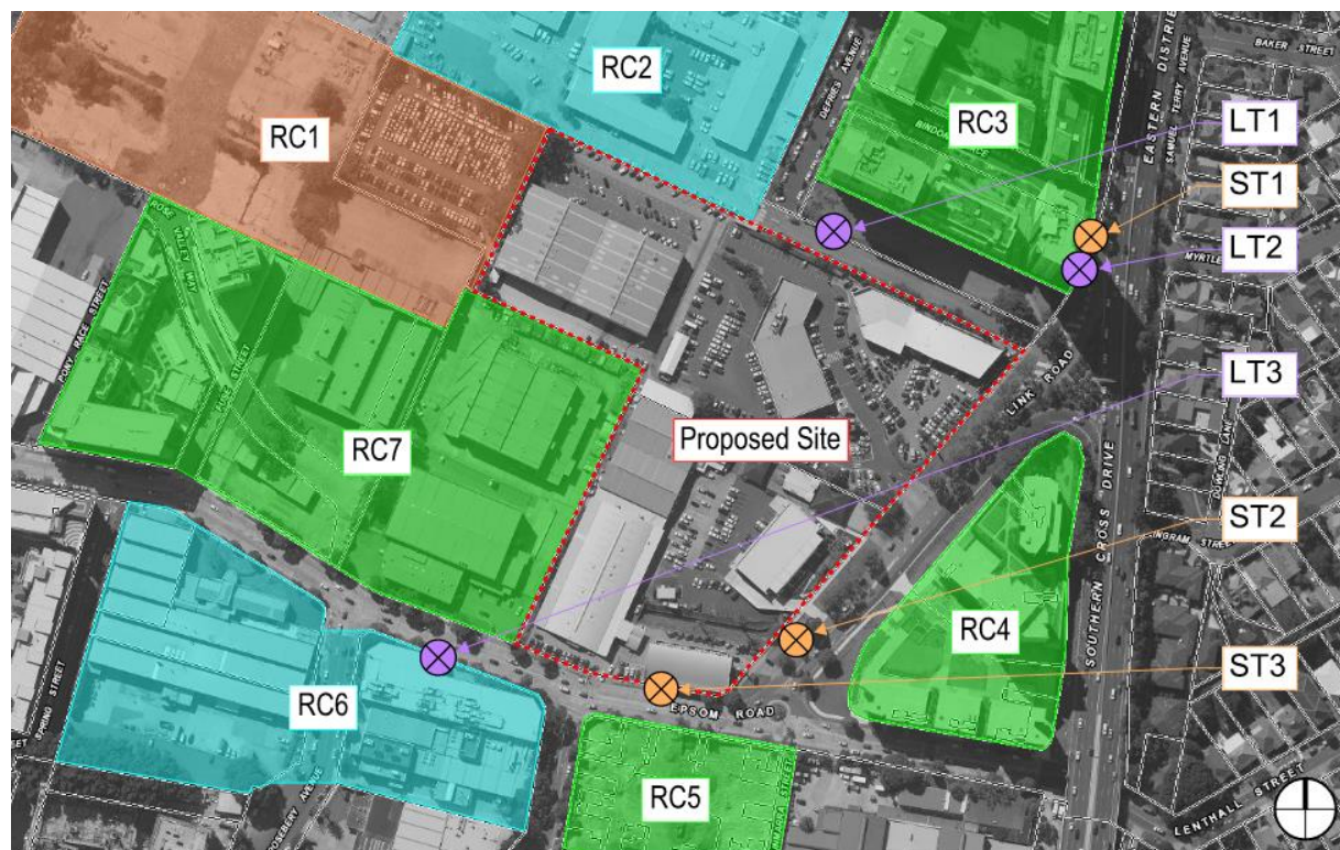
Figure 1: Acoustic site plan identifying the surrounding noise-sensitive receivers and noise monitoring locations
